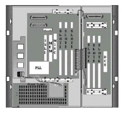
Figure 2-1 KSU With Expansion Type "A" Cabinet
